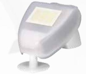
External Venetian Blinds around the building are controlled using the KNX Weather Station and a Sun-tracking algorithm in the Head-End Software. When the ambient light exceeds a defined threshold the blinds will tilt through a range of positions depending on their location on the façade. As a safety precaution should the wind speed exceed a defined level the blinds are retracted and held in the raised position until the wind reduces.
